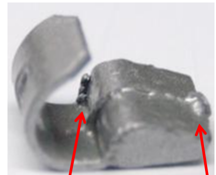
Excess Flash – Damage Potential & Fit Issues
